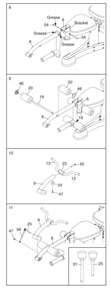
Slide a Safety Spotter (11) onto the Right Upright (5). Insert an Upright Pin (31) through the Safety Spotter and the Right Upright. Next, attach the Tether (58) on the Upright Pin to the Safety Spotter with an M4 x 16mm Screw (47).
